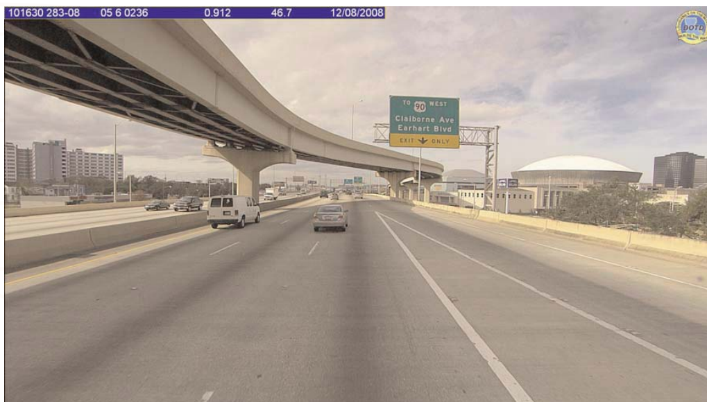
Pictured here: 1920 x 1080 pixel resolution (HDTV) Right-of-Way video image, with 90 degree horizontal field of view
