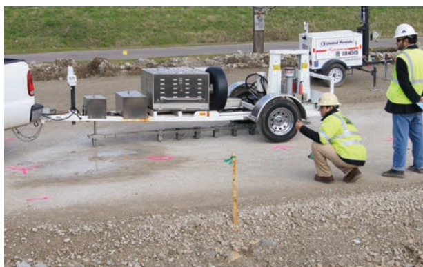
Pavement analysis using Falling Weight Deflectometer (FWD)
