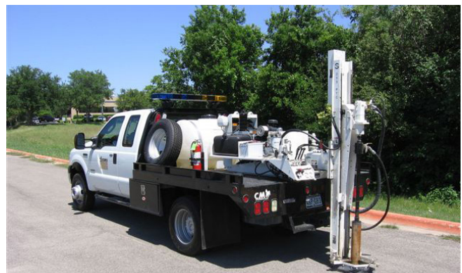
Coring is used to verify pavement thickness and to calibrate the GPR
